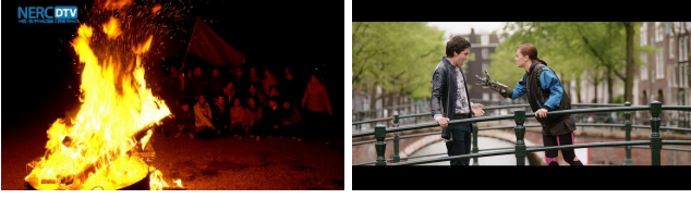
Figure 2. Examples of video content triggering false SCC in VVenC up to version 1.6.1. (left) Low lighting, saturation in JVET sequence Campfire [15], (right) black bars in 1080p movie Tears of Steel [16].
